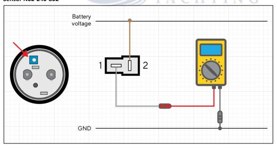
**Note:** if the multimeter leads are reversed, the measured current may be displayed negative (positive current is conventionally considered as flowing from the positive terminal to the negative one).
